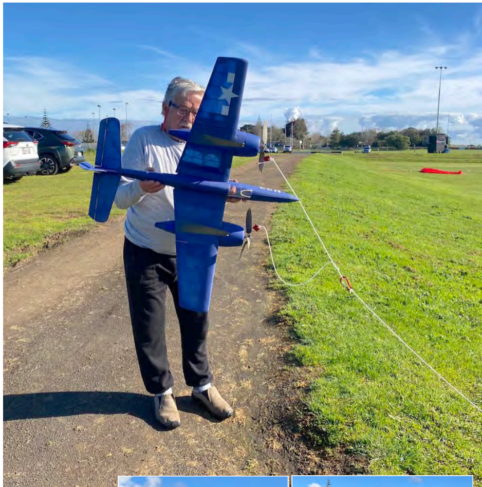
Upper: Don Spray with his rubber powered Grumman Tigercat. Cord to pull release pins for each motor are visible in this view. Propellers are contra-rotating.
